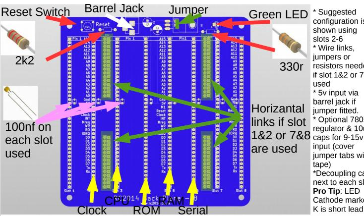
\* Suggested configuration is shown using slots 2-6 \* Wire links, jumpers or resistors needed if slot 1&2 or 7&8 used \* 5v input via barrel jack if jumper fitted. \* Optional 7805 regulator & 10uf input (cover jumper tabs with tape) \*Decoupling caps next to each slot Pro Tip: LED Cathode marked K is short lead
