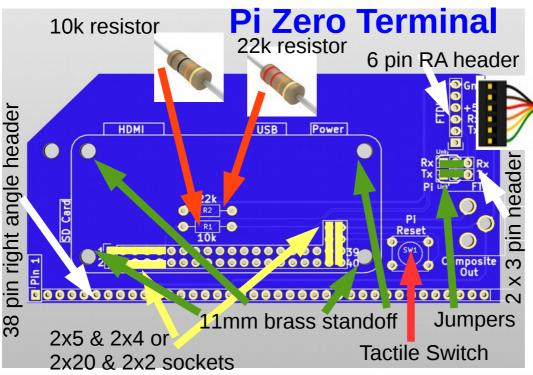
Solder pins, sockets, resistors & switch as indicated. Solder pins to the Raspberry Pi Zero. Tip: mate the sockets & pins first so they line up Use M3 bolts & standoffs to mount Pi Zero firmly. Set jumpers as indicated to use Pi as keyboard input and video output. (Set one or both to FTDI position to bypass the Pi) Use SD card supplied Pro Tip: Pi Zero holes may be tight fit. Use a
