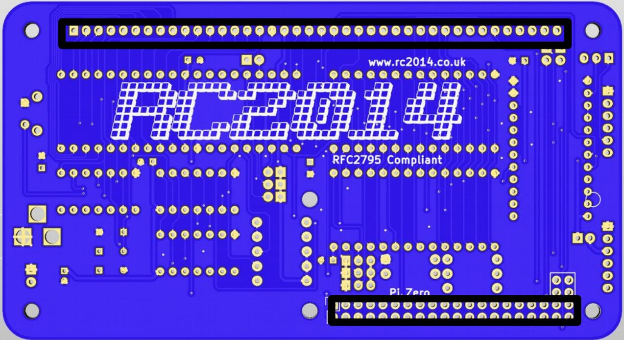
Fit 20x2 socket on underside if you plan to use Pi Zero
